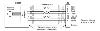
Figure 18 - SSI encoder cable connections
